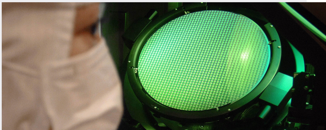
An engineer checks a 12-inch wafer, used for the fabrication of integrated circuits. (Credit: Sam Yeh / Staff, Getty Images)
